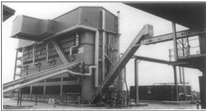
Figura 9: Sistem de reactor vertical (tip siloz)
